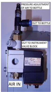
8. Instrument bridge air and water solenoid valve block:
